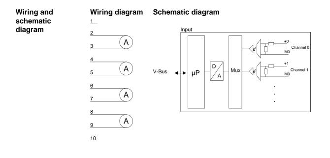
Wire break<br/>recognitionThe wire break recognition is always active. In case of a wire break res.<br/>when no encoder is connected, the LED of the according channel is turned<br/>on. The module has no diagnostic ability.
