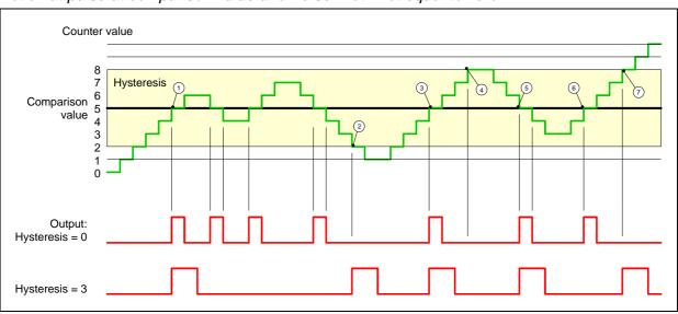
Action at pulse at comparison value and Pulse width not equal to zero
