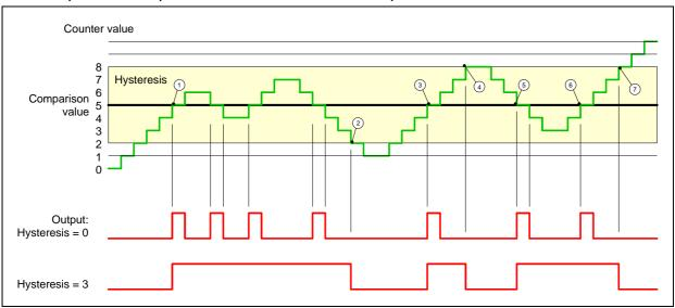
Action at pulse at comparison value and Pulse width equal to zero
