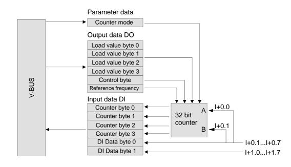
By writing *output data DO* to the module, you may preset a counter value with a *load value* as well as a *reference frequency*. The activation of this values takes place by means of the *control byte*.
