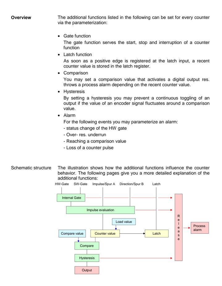
**Gate function** The counter is controlled via the internal gate (I-gate). The I-gate is the result of logic operation of hardware- (HW) and Software-gate (SW), where the HW-gate evaluation may be deactivated via the parameterization.
