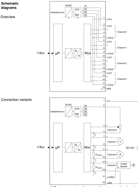
\*) During measuring the connection to ground is closed.
