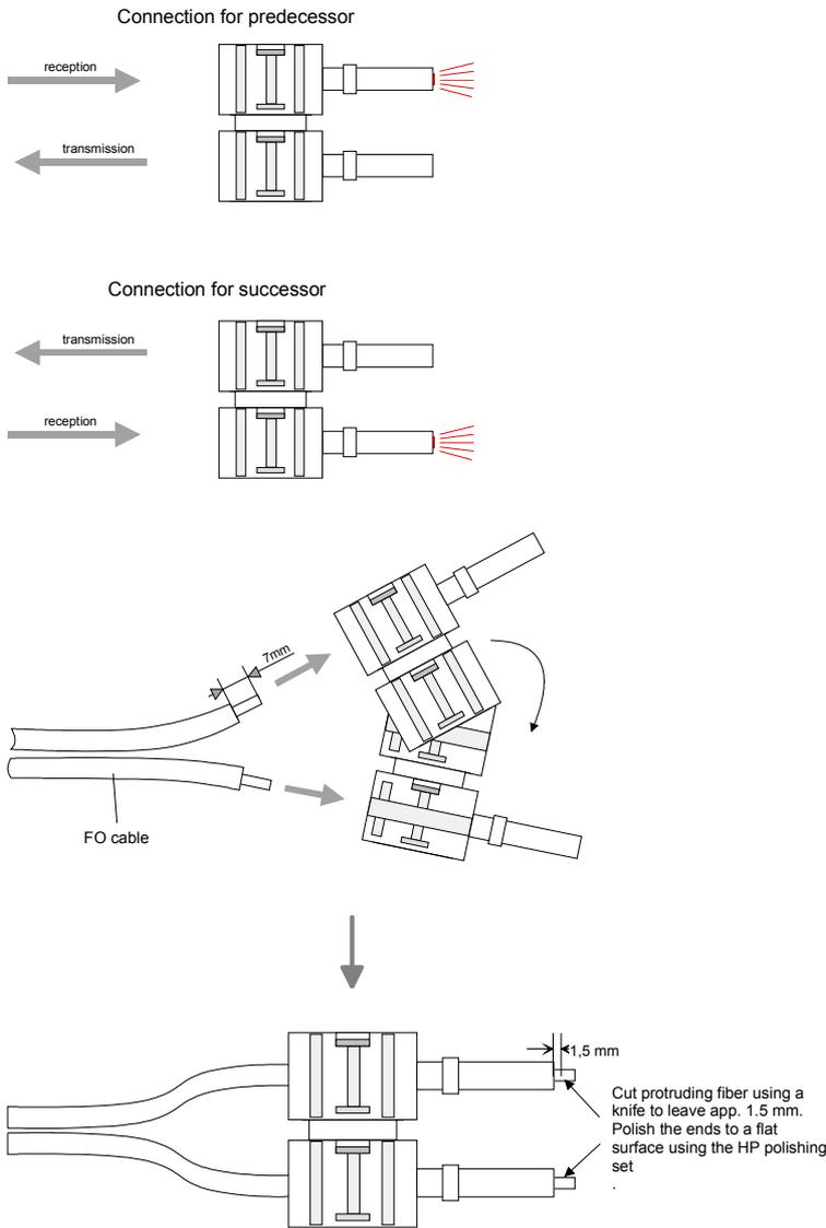
**Cutting and polishing the ends of the FO cable**
