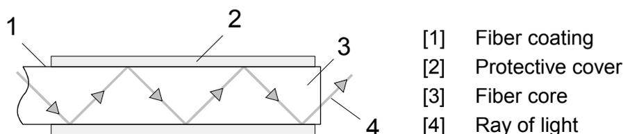
The fiber optic system employs pulses of monochromatic light at a wavelength of 650nm. If the fiber optic cable is installed in accordance with the manufacturers guidelines, it is not susceptible to external electrical interference. Fiber optic systems have a linear structure. Each device requires two lines, a transmit and a receive line (dual core). It is not necessary to provide a terminator at the last device.
