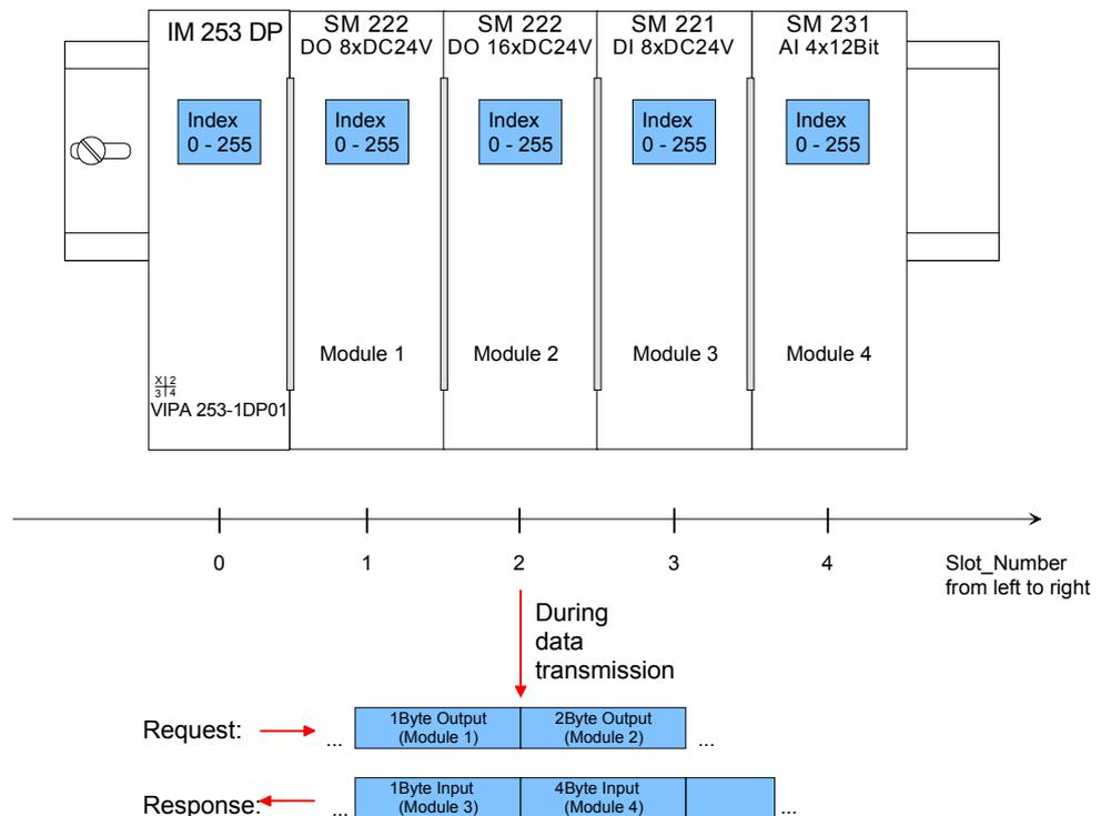
Each data block can be up to 244bytes. In the case of modular devices, the slot number is assigned to the modules. Compact devices are regarded as a unit of virtual modules. These can also be addressed with Slot\_Number and index.
