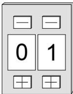
This address selector is used to configure the Profibus address for the DP slave. Addresses may range from 1 to 99. Addresses must be unique on the bus.
