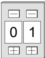
This address selector is used to configure the Profibus address for both DP slaves. Addresses may range from 1 to 99. Addresses must be unique on the bus.
