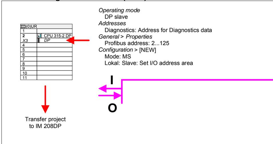
Hardware configuration superordinate master system (Siemens GSD required)
