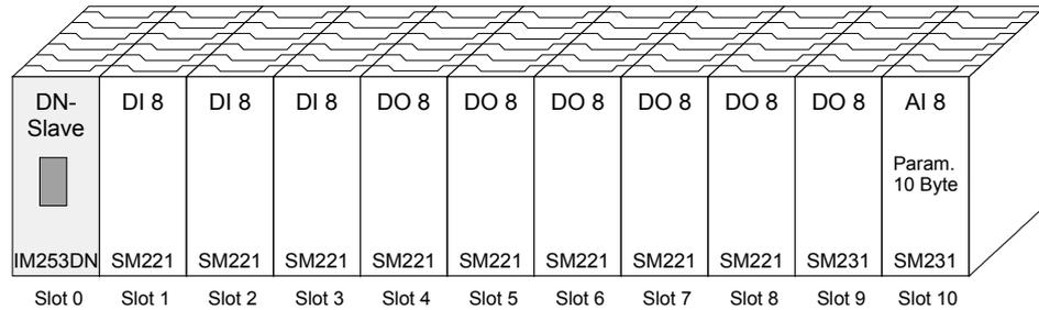
The example shows a DeviceNet coupler with 10 modules; however, the modules installed in plug-in locations 1 to 9 can not be configured.
