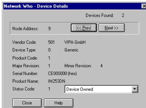
*Here you may display DeviceNet address (node address), the Vendor Code (in this case this is 501 for VIPA GmbH) and other internal information about every module on the bus.*
