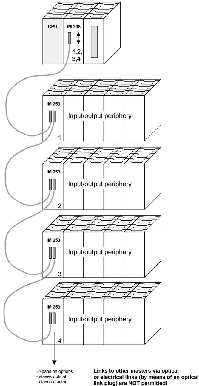
**Combination of optical and electrical Profibus**
