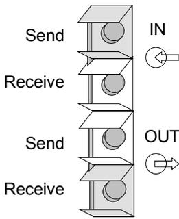
These connectors are provided for the optical waveguide between your Profibus coupler and the Profibus.
