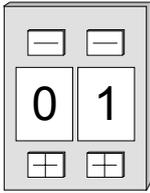
This address selector is used to configure the address for the bus coupler. Addresses may range from 1 to 99. Addresses must be unique on the bus. The slave address must have been selected before the bus coupler is turned on.
