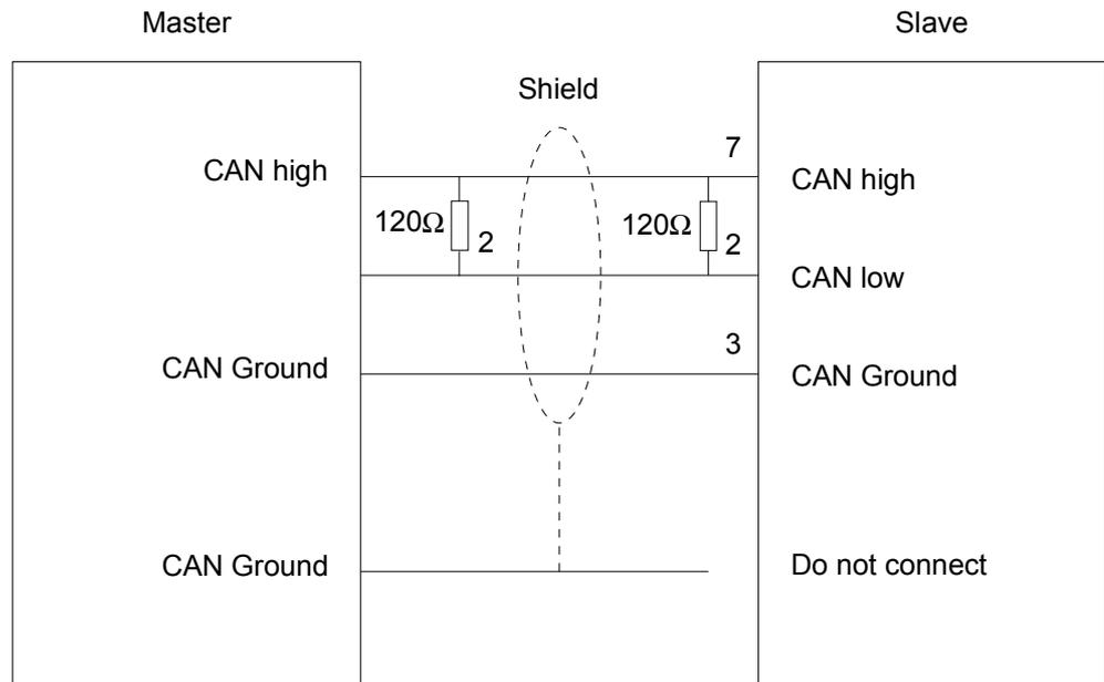
**Line termination** All stations on systems having more than two stations are wired in parallel. This means that the bus cable must be looped from station to station without interruptions.
