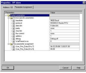
In this section of the parameterization you set the Modbus parameters.
