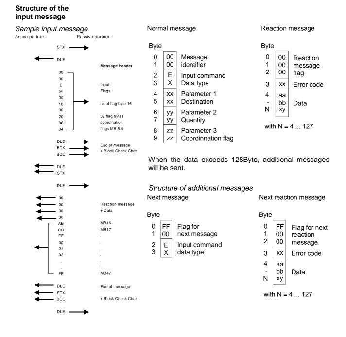
**Coordination flags** The coordination flag is set in the partner PLC in active-mode when a message is being received. This occurs for input as well as for output commands. When the coordination flag has been set and a message with this flag is received, then the respective data is not accepted (or transferred) and a reject message is sent (error code 32h). In this case the user has to reset the coordination flag in the partner PLC.
