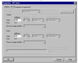
Here you may set from which address on the 16Byte for in- and output are stored in the CPU.
