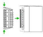
Install the connector on the module until it locks with an audible click.
