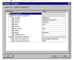
In this section of the parameterization you set the Modbus parameters.
