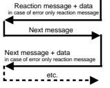
When the data quantity > 128 bytes subsequent messages are transmitted until all the data has been transferred.
