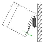
Insert the module that you are installing into the profile rail at an angle
