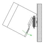
Insert the module that you are installing into the profile rail at an angle of 45 degrees from the top and rotate the module into place until it clicks into the profile rail with an audible click. The proper connection to the backplane bus can only be guaranteed when the module has properly clicked into place.
