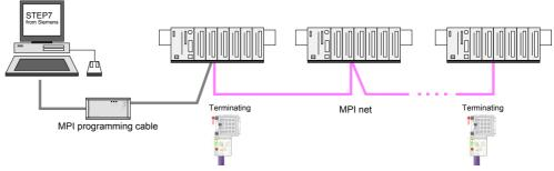
Transfer via Green Cable (serial communication)
