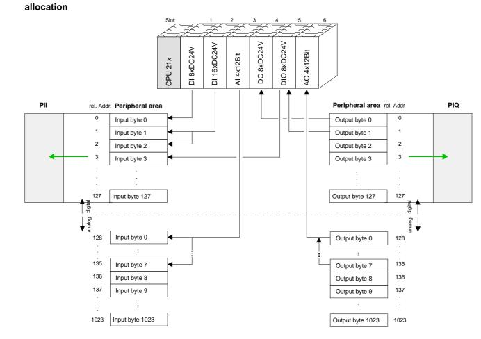
The following figure illustrates the automatic allocation of addresses:
