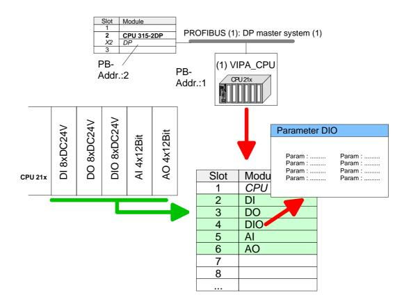
**Parameterization** For parameterization double-click during the project engineering at the slot overview on the module you want to parameterize. In the appearing dialog window you may set the wanted parameters.
