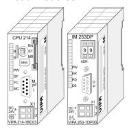
With a head module CPU respectively bus interface and DC 24V power supply are integrated to one casing. Via the integrated power supply the CPU respectively bus interface is power supplied as well as the electronic of the connected periphery modules
