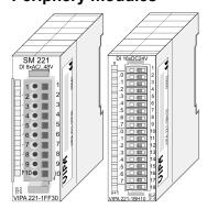
The modules are direct installed on a 35mm profile rail and connected to the head module by a bus connector, which was mounted on the profile rail before. The periphery modules are equipped with a 10pin respectively 18pin connector with recessed labelling. This connector provides the electrical interface for the signalling and supplies lines of the modules.
