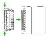
• Install the connector on the module until it locks with an audible click. For this purpose you press the two clips together as shown.
