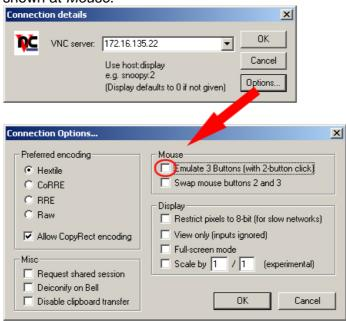
Enter the IP address of the Touch Panel at VNC server. With [OK] a VNC connection is established and the screen content of the Touch Panel is monitored within a window.
