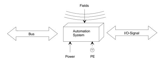
Interference is coupled into your system in different ways, depending in the propagation medium (conducted or not conducted) and the distance to the interference source.
