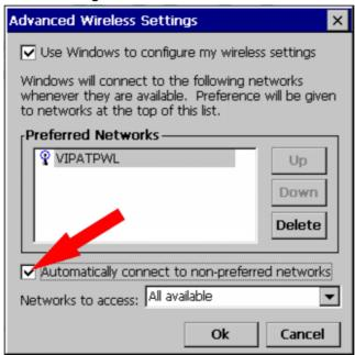
By activating of "Automatically connect to non-preferred networks" an automatically connection to the chosen network is established as soon as the network is available.
