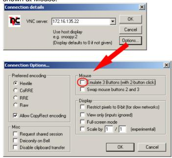
Enter the IP address of the Touch Panel at VNC server. Click on [OK] and enter the password vipatp. Now a VNC connection is established and the screen content of the Touch Panel is monitored within a window.
