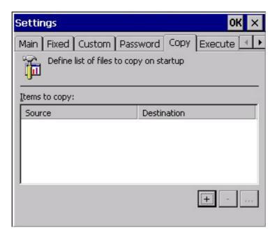
Here with the startup of the panel files may be copied e.g. from flash disk to Windows<sup>®</sup>.
