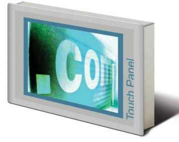
**TP 606C CAN** 606-3B1F0 The VIPA Touch Panel is a compact and modular embedded PC based on Windows<sup>®</sup> CE. Besides of the extensive Windows<sup>®</sup> CE functions the Touch Panel offers varied communication possibilities. Here the Touch Panel can simply be configured, controlled and remoted. By including a selectable HMI/SCADA runtime the Touch Panel is particularly suitable for monitoring and controlling of process cycles.
