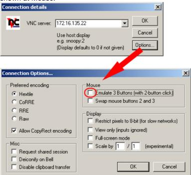
Enter the IP address of the Touch Panel at VNC server. With [OK] a VNC connection is established and the screen content of the Touch Panel is monitored within a window.
