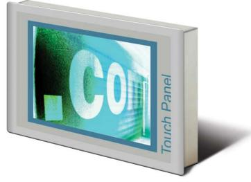
**TP 605LQS** 605-1BL00 The VIPA Touch Panel is a compact and modular embedded PC based on Windows<sup>®</sup> CE. Besides of the extensive Windows<sup>®</sup> CE functions the Touch Panel offers varied communication possibilities. Here the Touch Panel can simply be configured, controlled and remoted. By including a selectable HMI/SCADA runtime the Touch Panel is particularly suitable for monitoring and controlling of process cycles.
