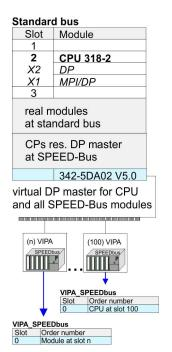
For the employment of the I/O modules at the SPEED-Bus the inclusion via the GSD-file from VIPA in the hardware catalog is required.
