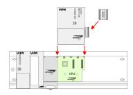
If also standard modules shall be plugged, take a bus coupler and click it at the CPU from behind like shown in the picture. Plug the CPU between the triangular positioning helps to the slot marked with "CPU SPEED7" and pull it down.
