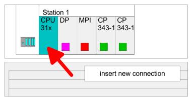
⇒ Via the dialog window you may set the parameters for a connection. The parameters ID and LADDR are required for the usage on the blocks AG\_SEND res. AG\_RECV. With deployment of Siemens S7 connections the parameter *ID* is to be passed to the respective FB/SFB VIPA handling blocks.
