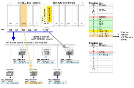
The according module is to be taken from the hardware catalog to slot 0 of VIPA\_SPEEDBUS.
