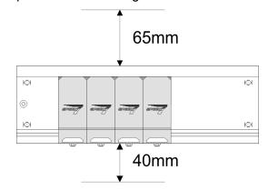
2. Connect the profile rail with the protected earth conductor. The minimum cross-section of the cable to the protected earth conductor has to be 10mm<sup>2</sup>.
