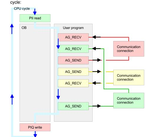
The FC blocks with concerning communication connection are summed up by colour. Here you may also see that your user application may consist of any number of blocks. This allows you to send or receive data (with AG SEND res. AG RECV) event or program driven at any wanted point within the CPU cycle. You may also call the blocks for one communication connection several times within one cycle.
