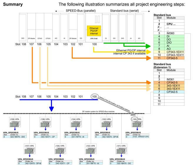
The according module is to be taken over from the HW catalog of VIPA\_SPEEDBUS on slot 0.
