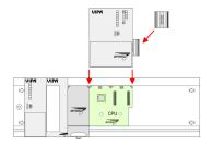
If also standard modules shall be plugged, take a bus coupler and click it at the CPU from behind like shown in the picture. Plug the CPU between the triangular positioning helps to the slot marked with "CPU SPEED7" and pull it down.
