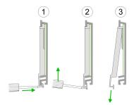
Dismantle the according protection flaps of the SPEED-Bus slot with a screw driver (open and pull down).
