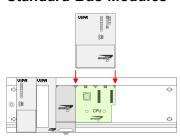
To deploy the SPEED7-CPU exclusively at the SPEED-Bus, plug it between the triangular positioning helps to the slot marked with "CPU SPEED7" and pull it down.
