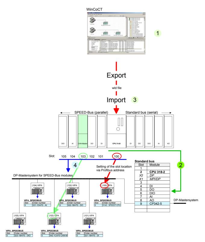
The according module is to be taken over from the HW Catalog of VIPA\_SPEEDBUS to slot 0.
