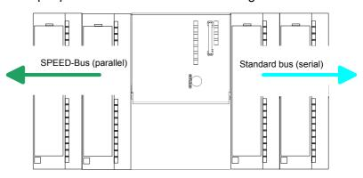
Serial The single modules are directly installed on a profile rail and connected via the backplane bus coupler. Before installing the modules you have to clip Standard bus the backplane bus coupler to the module from the backside. The backplane bus coupler is included in the delivery of the peripheral modules.
