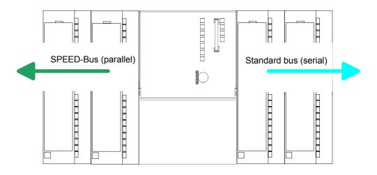
**CPU 31xS** The System 300S series consists of a number of CPUs. These are programmed in STEP<sup>®</sup>7 from Siemens. For this you may use WinPLC7 from VIPA or the Siemens SIMATIC manager.
