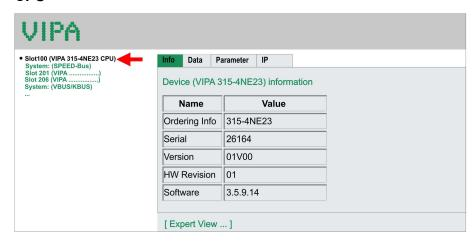
Here order number, serial number and the version of firmware and hardware of the CPU are listed. [Expert View] takes you to the advanced "Expert View".
