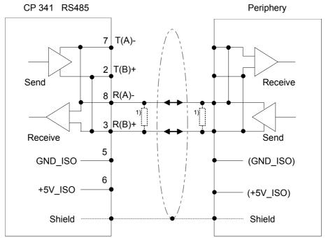
In the case of cables >50m you have to solder in a terminating resistor of approx.  $330\Omega$  on the receiver for data free traffic.
