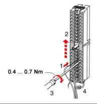
Fix the cable binder for the cable bundle.
