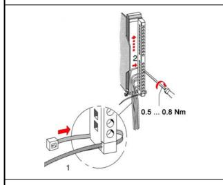
Put the included cable binder around the cable bundle and the front connector.
