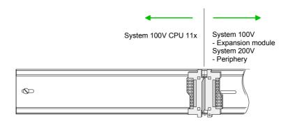
Plug in your System 100V CPU 11x until it snaps into position at the right side of the bus coupler.
