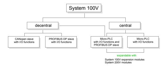
**Central system** The central system is built of one CPU and integrated I/O-functions. The CPU is instruction compatible to the S7-300 from Siemens and may be programmed and projected by means of S7 programming tools from Siemens and VIPA via MPI.
