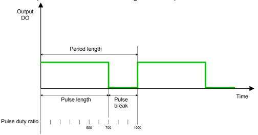
Period length = time base x period Pulse length = (period length / 1000) x pulse duty ratio Pulse break = period length - pulse length
