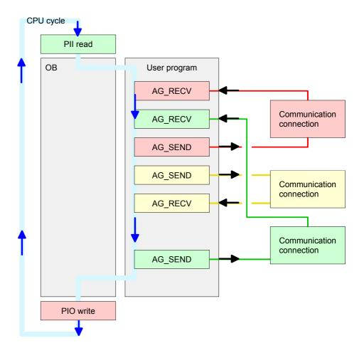
The FC blocks with concerning communication connection are summed up by color. Here you may also see that your user application may consist of any number of blocks. This allows you to send or receive data (with AG\_SEND res. AG\_RECV) event or program driven at any wanted point within the CPU cycle.
