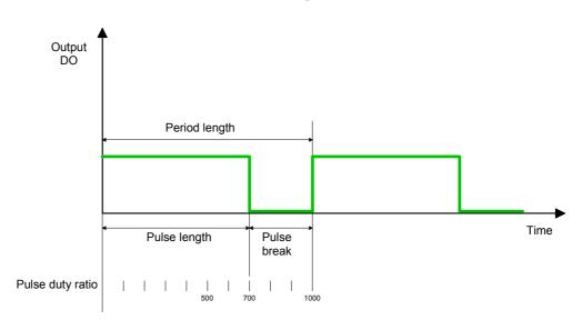
Period length = 1 / frequency Pulse length = (period length / 1000) x pulse duty ratio Pulse break = period length - pulse length
