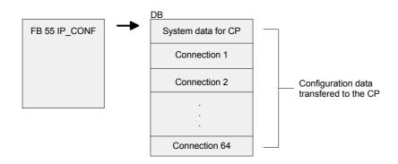
The configuration DB may be loaded into the CP at any time.
