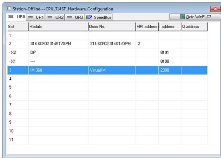
5. For transferring the hardware configuration you must at first specify the mode of the transfer. This must be adjusted in the menu bar under “Target:”. Then execute the transfer of the hardware configuration in the menu bar.
