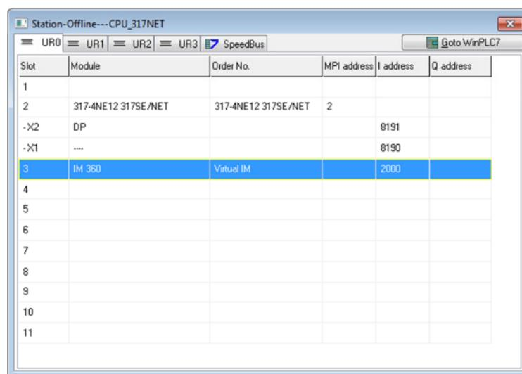
5. Insert beginning at slot 4 all modules, which are located on the standard bus to the right of the CPU. Mark the line and insert them by double click on the module. In this HTD example 1x 16Bit digital input module und 1x 16Bit Digital output module ( under: **S7-300\_DI-300** and **S7-300\_DO-300** ) were used.
