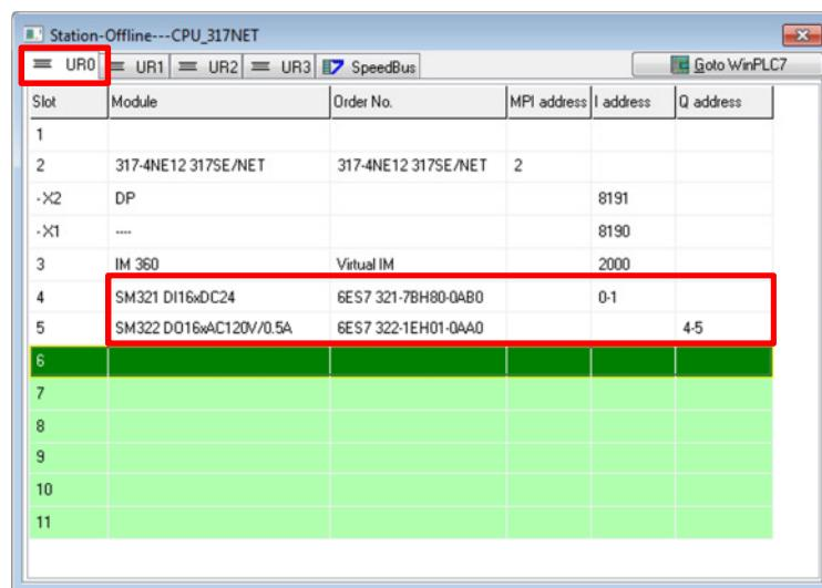
6. Shift to the register card „Speed Bus“. Here you must insert all external CPs, which are located to the left of the CPU on the SPEED Bus. In this HTD example 2x DP-Master (directory: **S7-300 → Speed-Bus-Module -> 342-1DA70 DP Master**) and 1x Ethernet CP (directory: **S7-300 -> Speed-Bus-Module -> 343-1EX71 Ethernet-CP**) were used. Now the station should look like the following picture:
